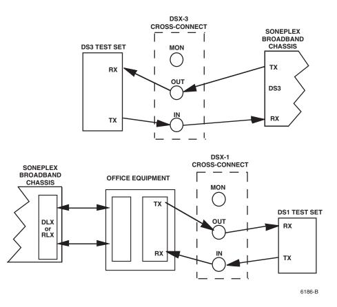
Figure 522-1. Test Setup
